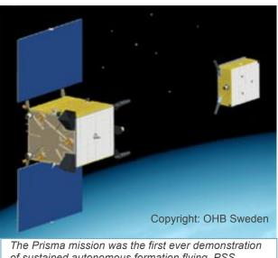
of sustained autonomous formation flying. PSS designed Prisma's safe orbit guidance algorithms.
