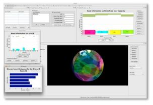
displays beam footprints, users and RFI sources, while the bar charts illustrate capacity and demand for selected users, beams and channels.
